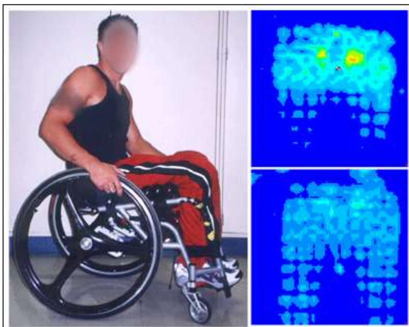
Figure 6: Pressure maps show pressure before (top) and after (bottom) adding a wedge to the patient's seating, improving distribution of pressure.
