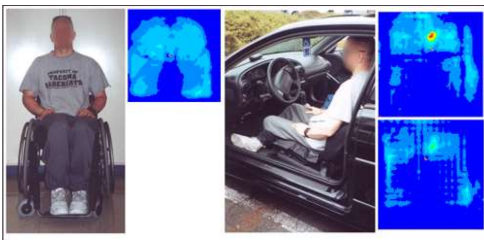
Figure 9: Pressure map in the wheelchair is good. In the car seat there is a red high pressure area (top right) that disappears when a cushion is added (bottom right).
