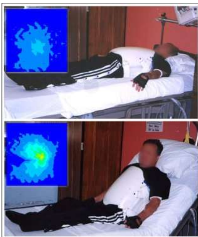
Figure 8: Pressure map while lying flat in bed is good (top) but gets worse when back rest is elevated.
