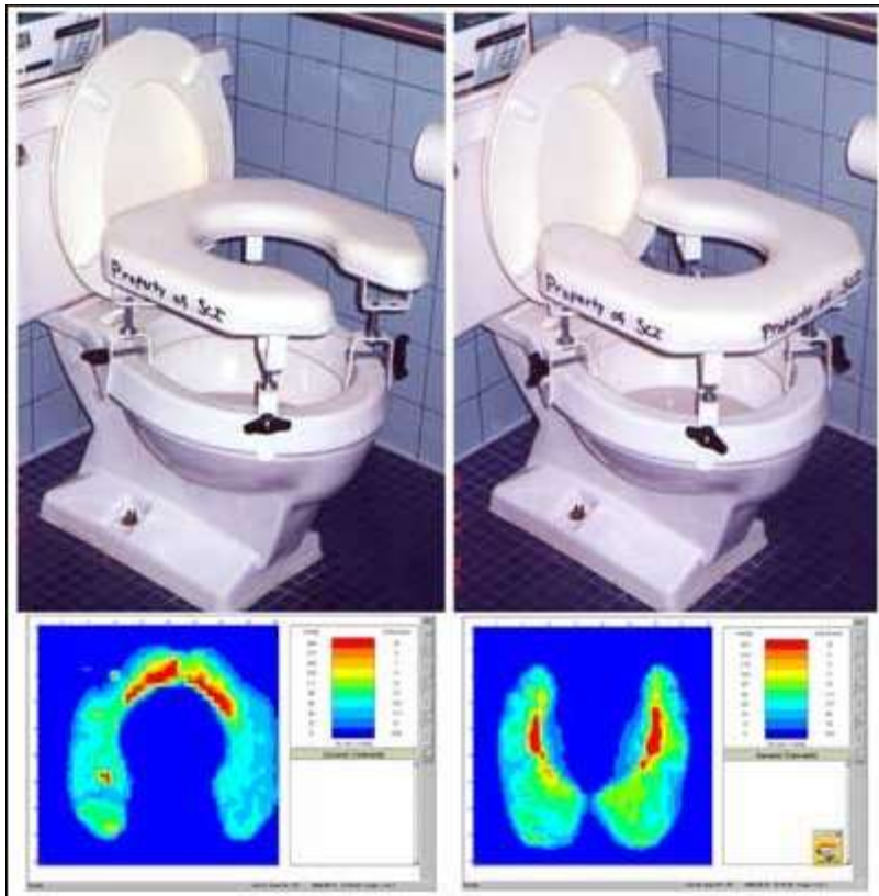
Figure 7: On the left the high pressure areas are located in the tailbone area, where the patient had an active wound. Turning the toilet seat around (right) takes pressure off the wound.
